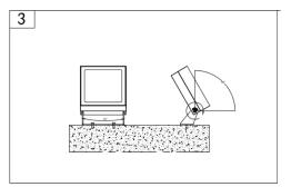
3. Notes: The fixture must get reliable connection with the mounting surface, any screws in the lamps should not be arbitrarily loosed. There is no special requirement on the installation direction.
